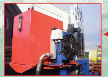
Integral conveyor hydraulic system with thermostatically controlled cooling system.
