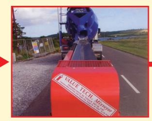
Belt drive motor is recessed in discharge canopy.
