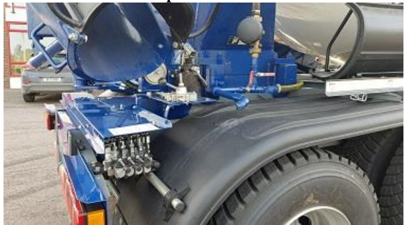
Mixer Manual Control positioned near tele-chute control.
