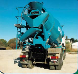
The Hydraulic Demountable System, enables quick and easy attaching & detaching from Truck Mixer.
